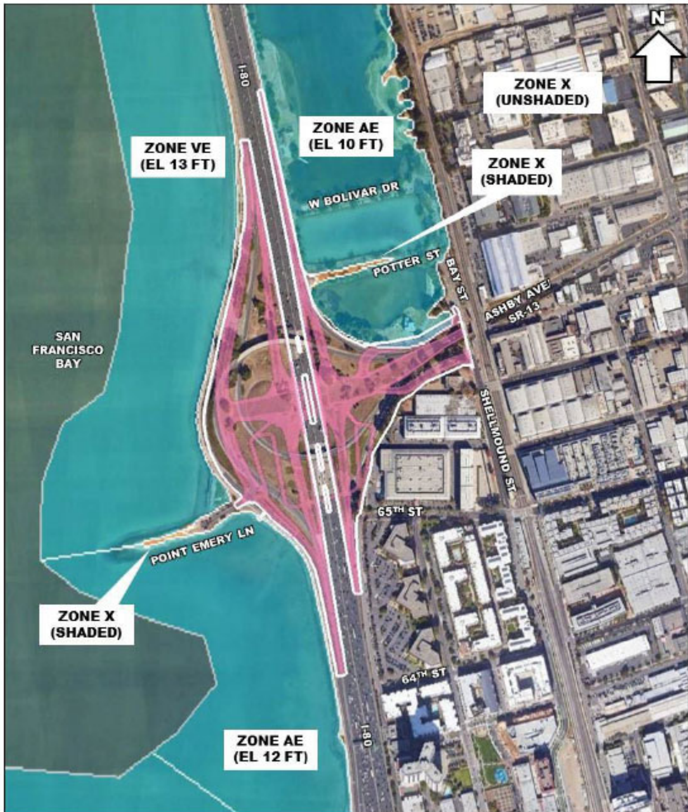
FEMA FLOODPLAIN ZONES AND BUILD ALTERNATIVE 1 (SPUI)
