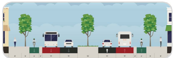
Proposed Typical Mid-Block Cross-section
