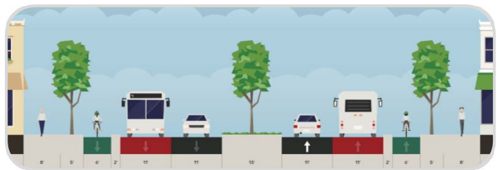
Proposed Typical Mid-Block Cross-section
