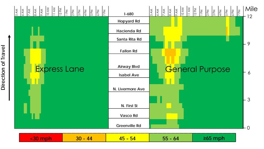
Express Lane speeds are generally above 50 mph at all times throughout the corridor, which is comparatively better than general purpose lanes speeds, which average 40 mph during the morning peak near Fallon Road. Average corridor speed differential range from 4-8 mph depending on time of day.
