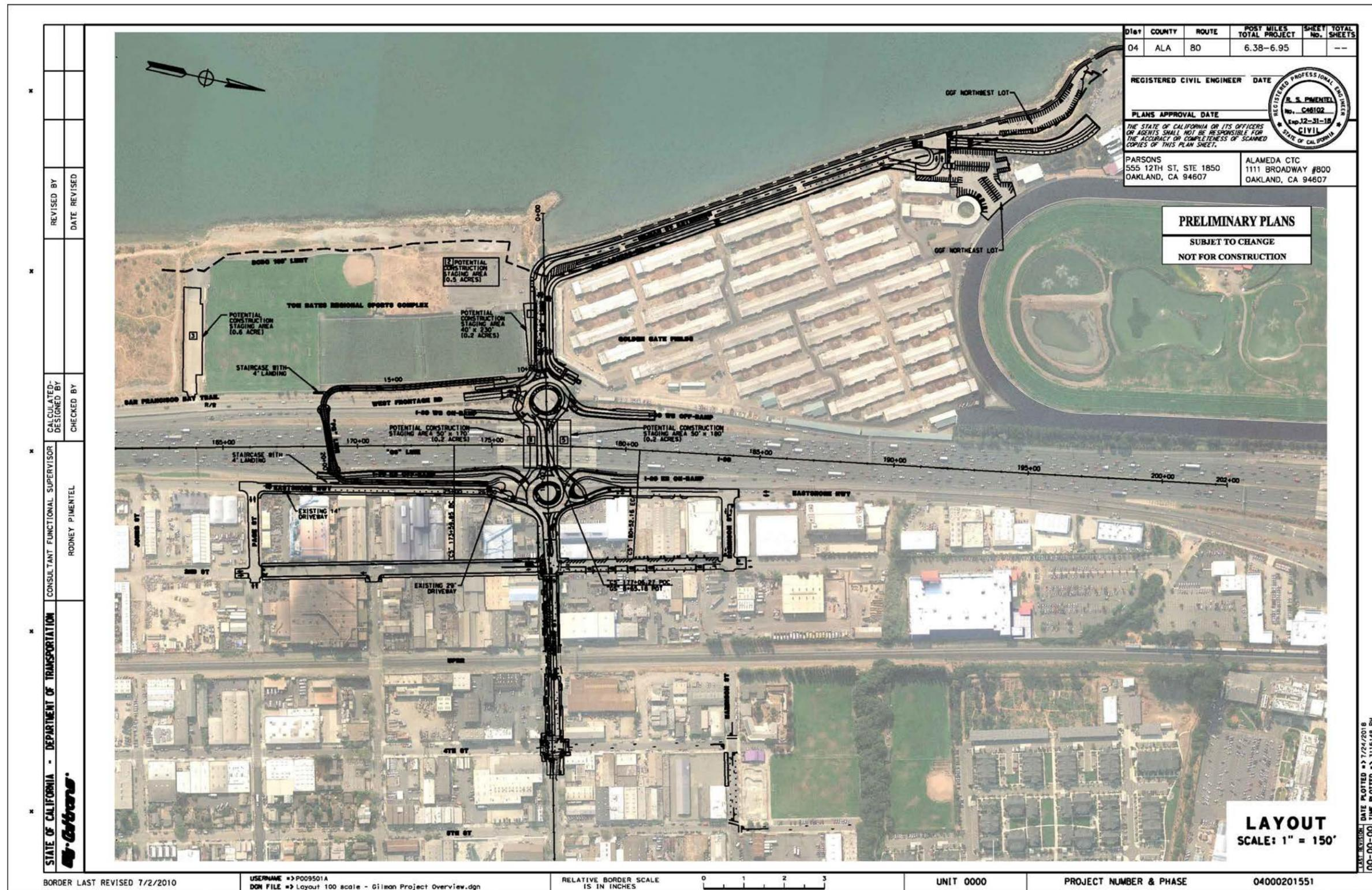
Figure 1-3: Roundabout Alternative
