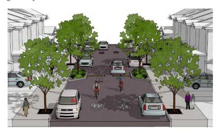
• Class IV: <u>Separated bike lanes</u>. These bikeways are for the exclusive use of bicyclists, separated from both automobile and pedestrian traffic. Separation can be provided by grade separation, an on-street parking lane, flexible posts, or inflexible barriers (e.g., pre-cast curb, bollards). Separated bike lanes are generally an urban treatment.
