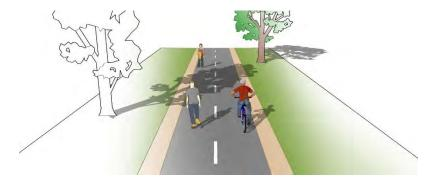
• Class II: <u>Bike lanes</u>. These bikeways exist on roadways as spaces for the exclusive use of bicyclists. Drivers may enter the bike lane to make a turn or to access curbside parking. Bike lanes may also be buffered with wide striping where space is available to provide greater separation from traffic.
