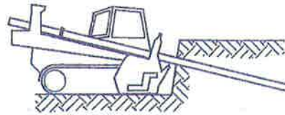
STEP 2. DRILL NAIL HOLE
