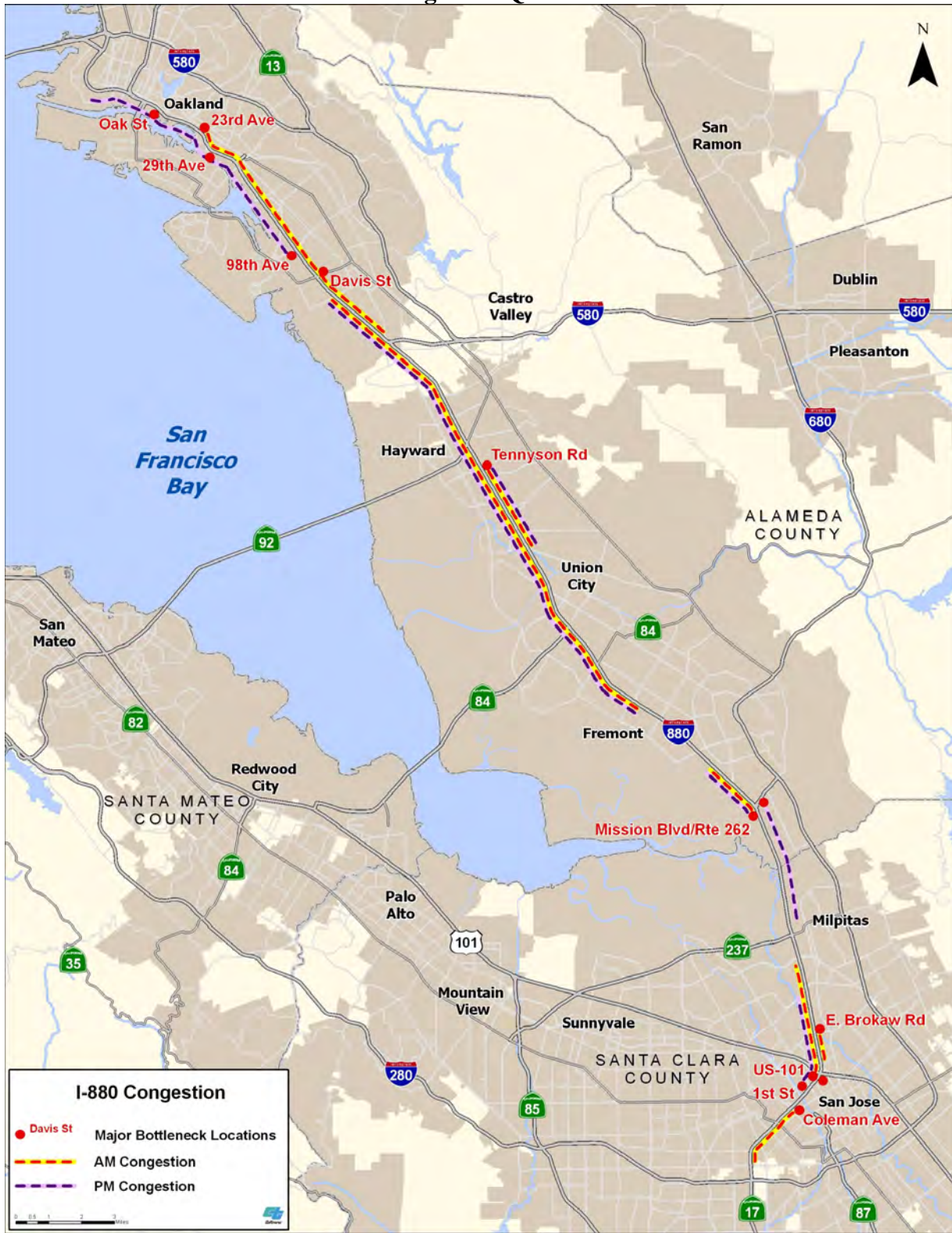
Figure ES2. Bottlenecks and Congestion Queues on I-880 Corridor (2004-07).
