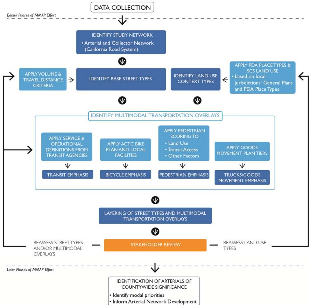
Figure 1: Multimodal Arterial Plan Typology Framework Process Diagram
