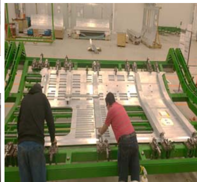
13 th Vehicle – Side Wall Welding
