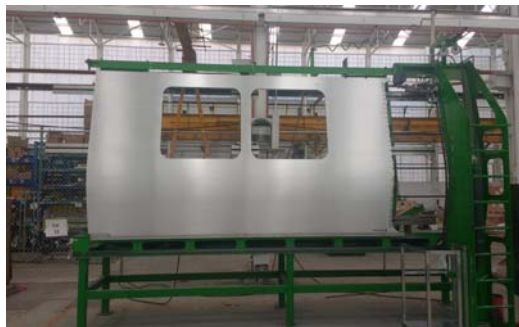
Side Wall Brushing
