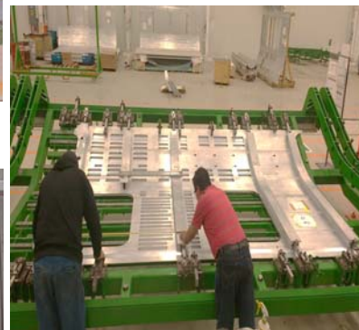
13 th Vehicle – Side Wall Welding
