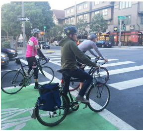
Bike box pavement markings
