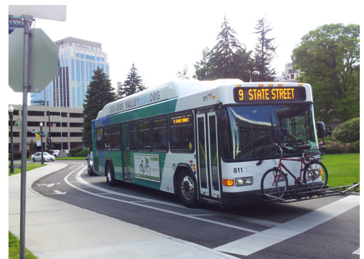
Bike lane with striped buffer
