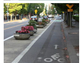
Bike lanes protected by on-street parking
