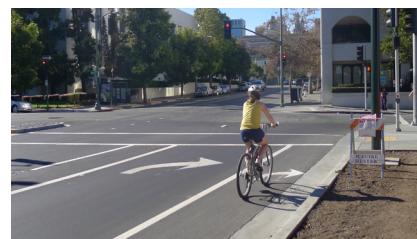
Bicycle right-turn lane adjacent to right-turn lane for vehicles
