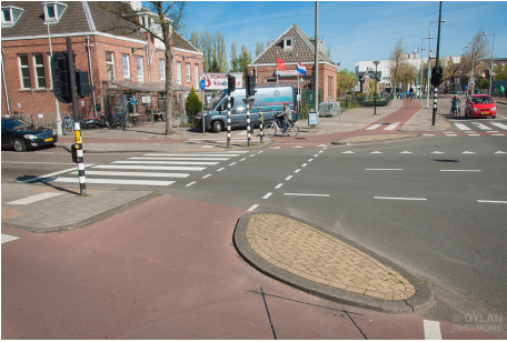
Protected intersection with colored pavement
