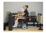
BusBuddy compares itself with rear-facing restraints in reduction of securement time and independence of use, while at the same time allowing the rider to face forward. It would not be necessary to change the vehicle specifications adopted under the ADA to make use of the BusBuddy system. On the prototype, a yellow bar comes down in front for the rider to hold onto. A red bar comes down on the side to prevent tipovers. The next step is testing of the prototype.
