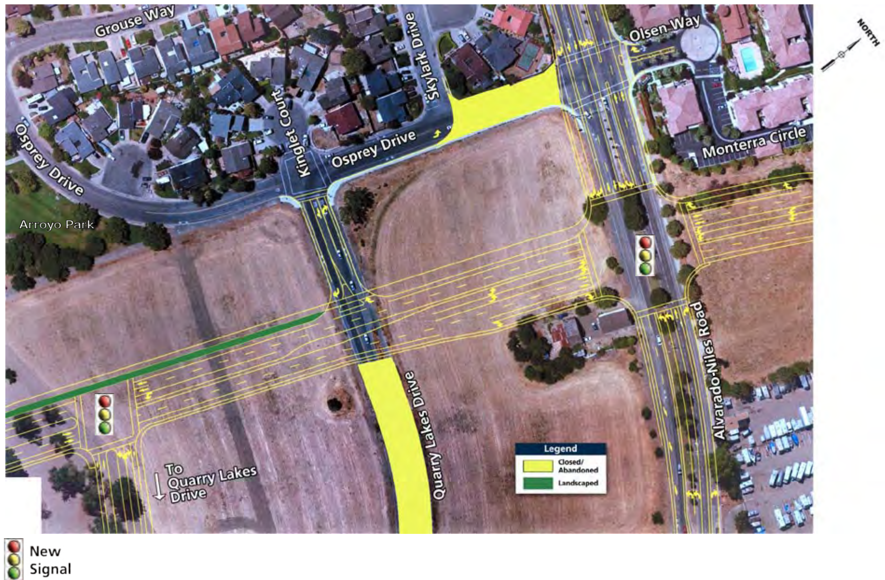
Figure 2-7a Proposed Quarry Lakes Drive Realignment Option 1: Three-Way Intersection ACTA East-West Connector Project
