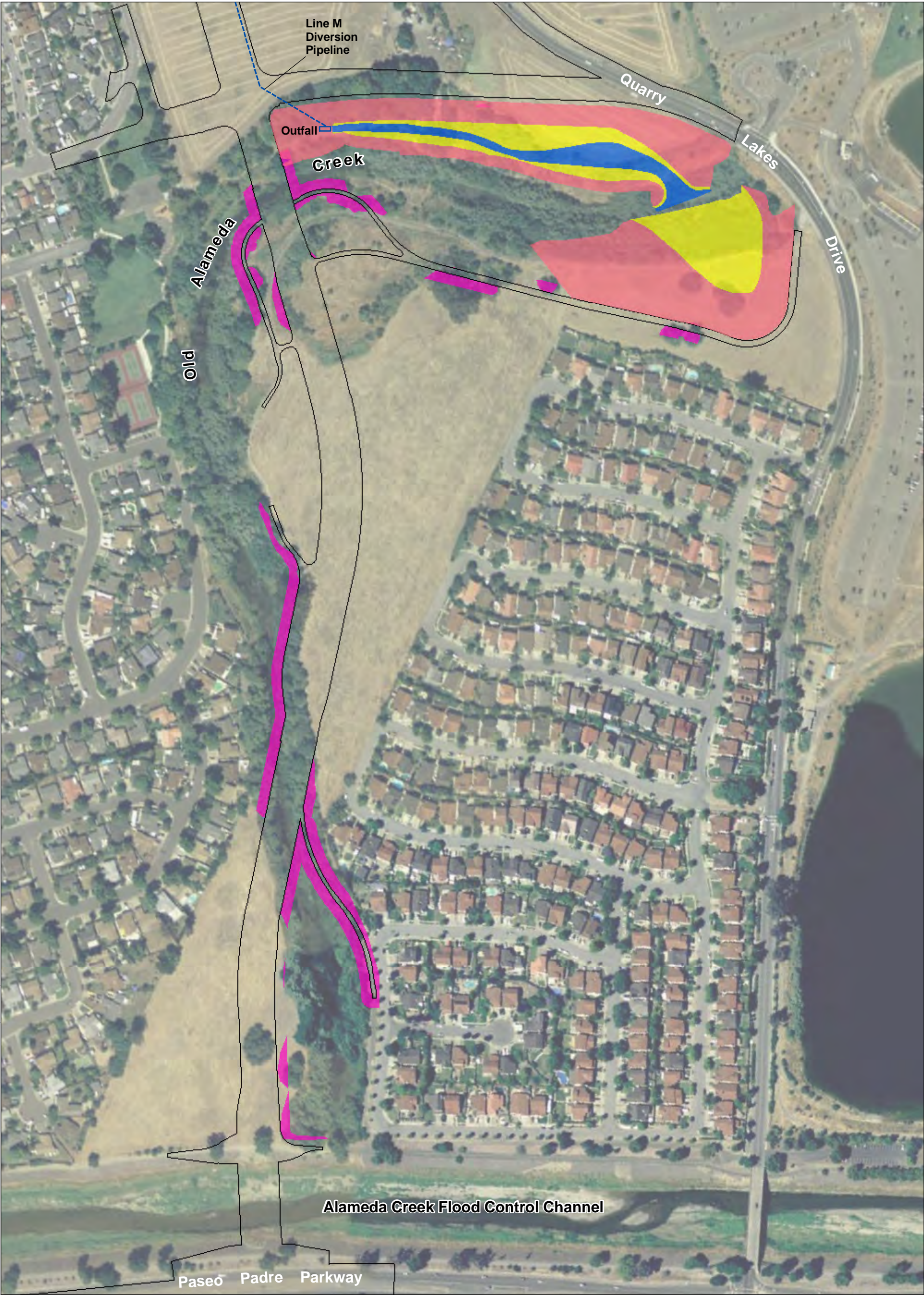
Figure 3.3-3 Draft Wetlands Mitigation Plan and Riparian Vegetation Restoration ACTA East-West Connector Project
