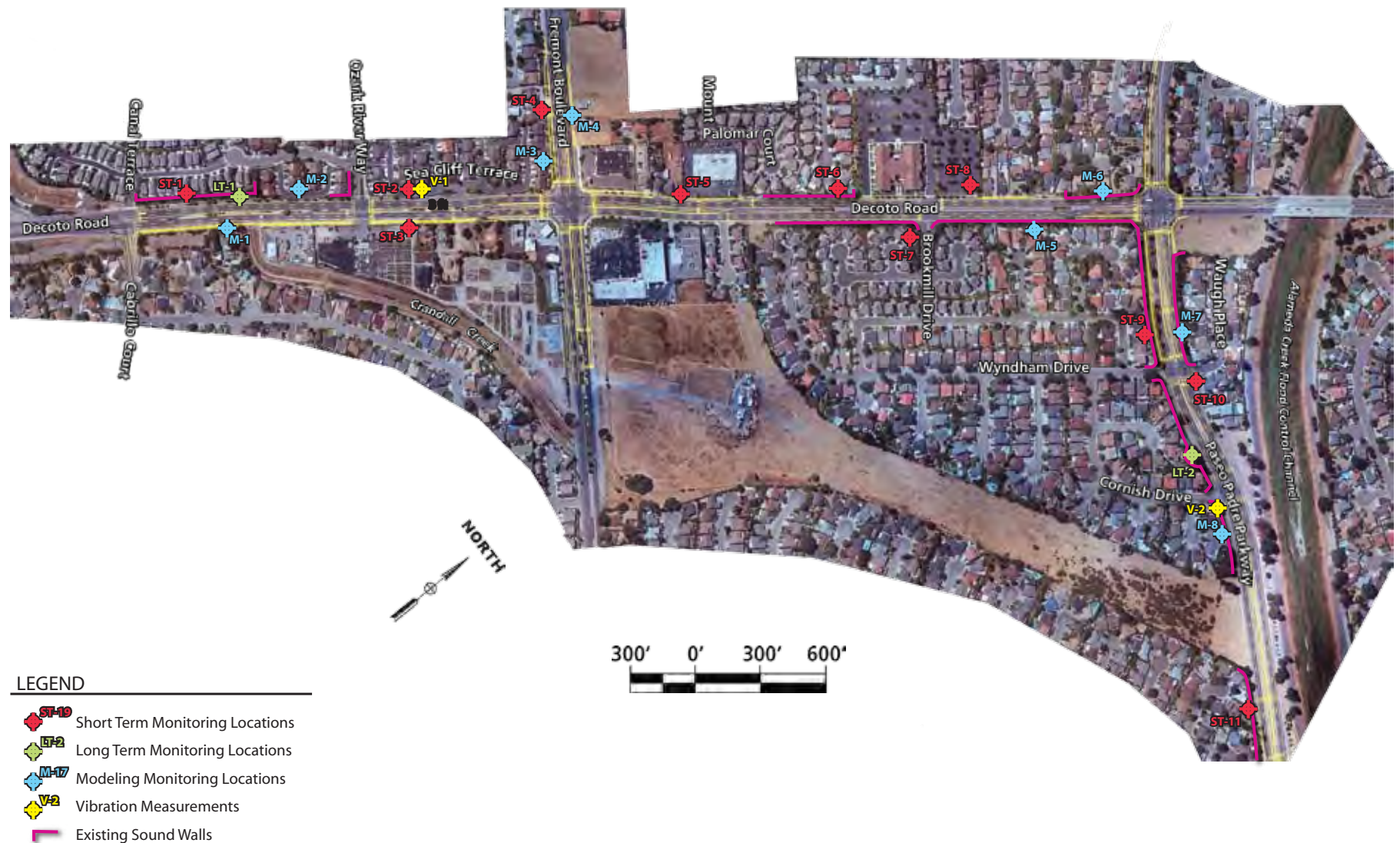
Figure 3.9-1a Noise Measurement Locations ACTA East-West Connector Project
