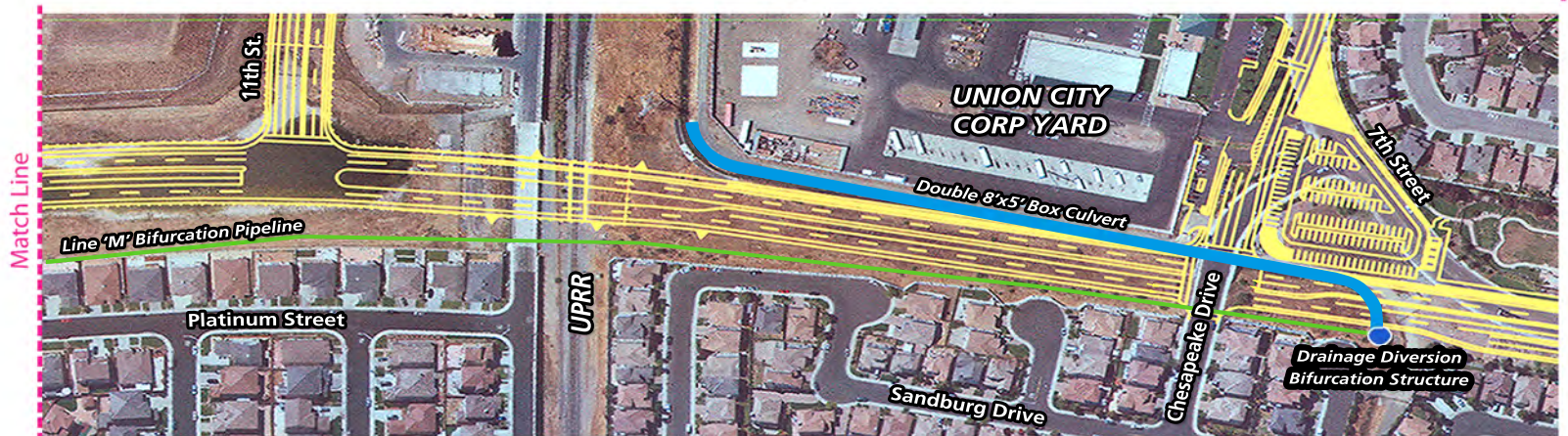
Figure 2-10 Proposed Line M Channel and Diversion Pipeline ACTA East-West Connector Project
