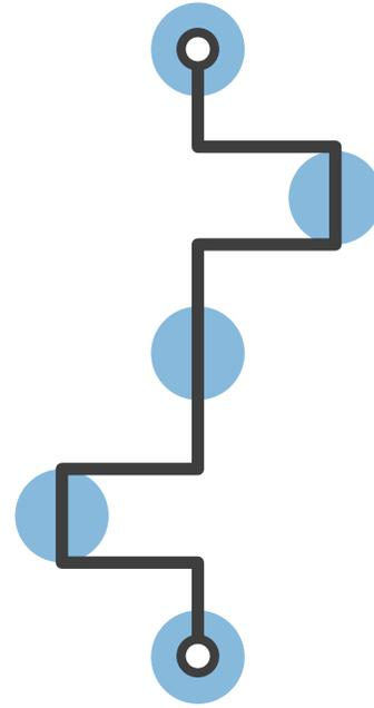
**Figure 2.1** - Poor transit geography forces a choice between providing a slow, meandering route or one that bypasses key destinations (figure adapted from Trans Link).
