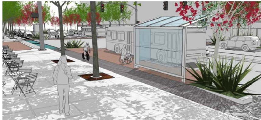
Far-Side Bus Stop with Bulbout, ADA Compliant Loading Platform, Bus Shelter, Bench and Class 4 Protected Bicycle Lane (Image source: San Pablo Avenue Specific Plan )
