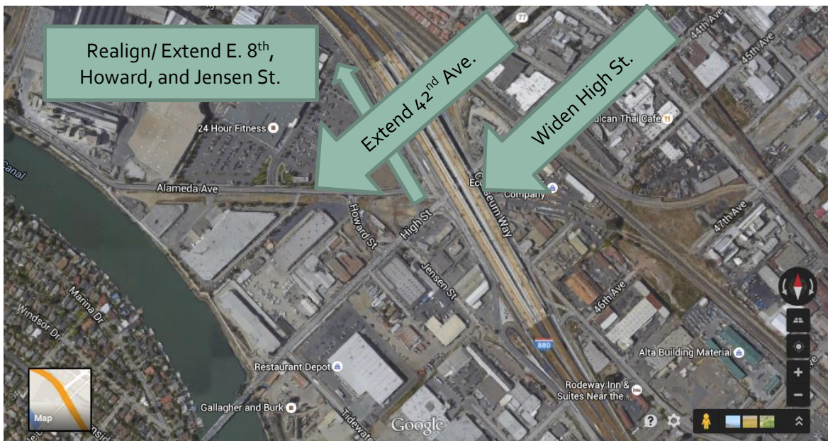
Figure 6.5 I-880/High St Interchange Improvements Project Location
