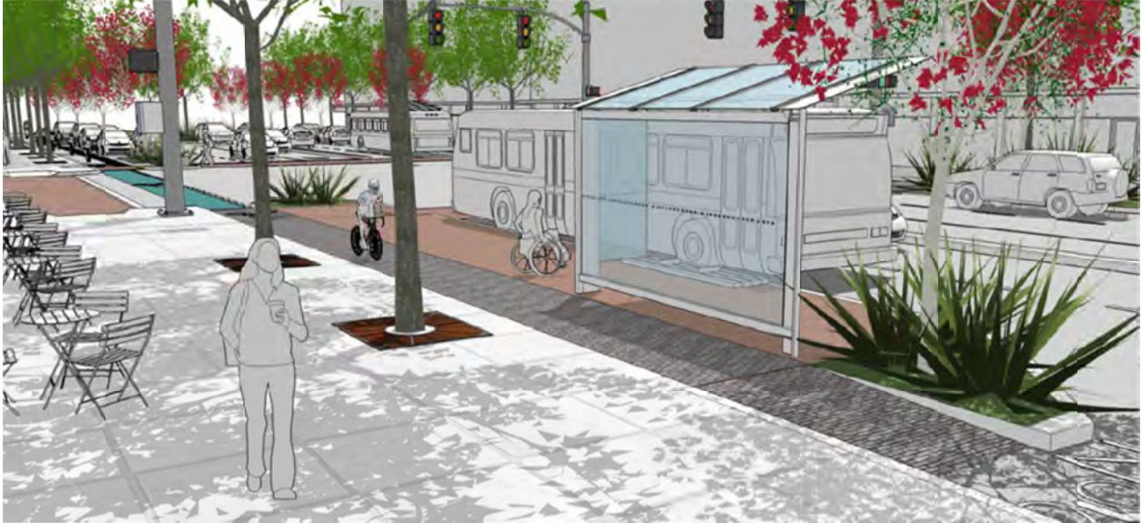
Far-Side Bus Stop with bulb-out, ADA-compliant loading platform, bus shelter, bench and Class 4 protected bicycle lane
