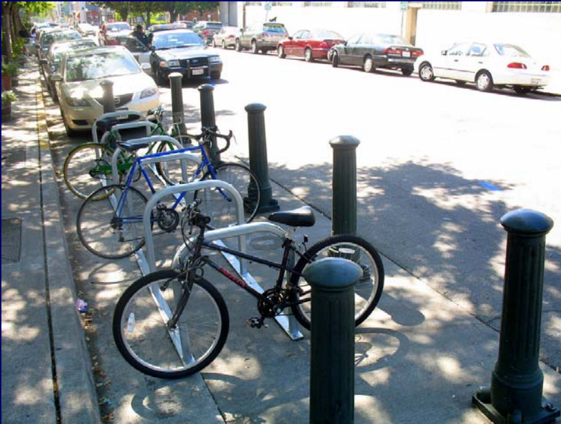
Parallel Parking: In-street bike parking delineated by heavy-duty architectural bollards on concrete pad
