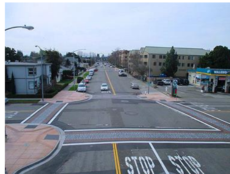
West Juana Pedestrian Improvements: Bulb outs and stamped crosswalks
