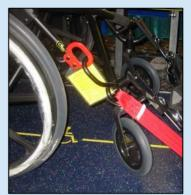
Overwhelming support for ANSI/RESNA "WC-19" standard ('transit option' consisting of permanent brackets or loops on mobility aids for the attachment of vehicle tie-down equipment.)
