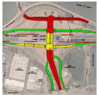
Figure 1.5-18 Roundabout Option A
