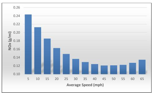
Figure 2.2-2 NO<sub>x</sub> Emissions Based on Vehicle Speed
