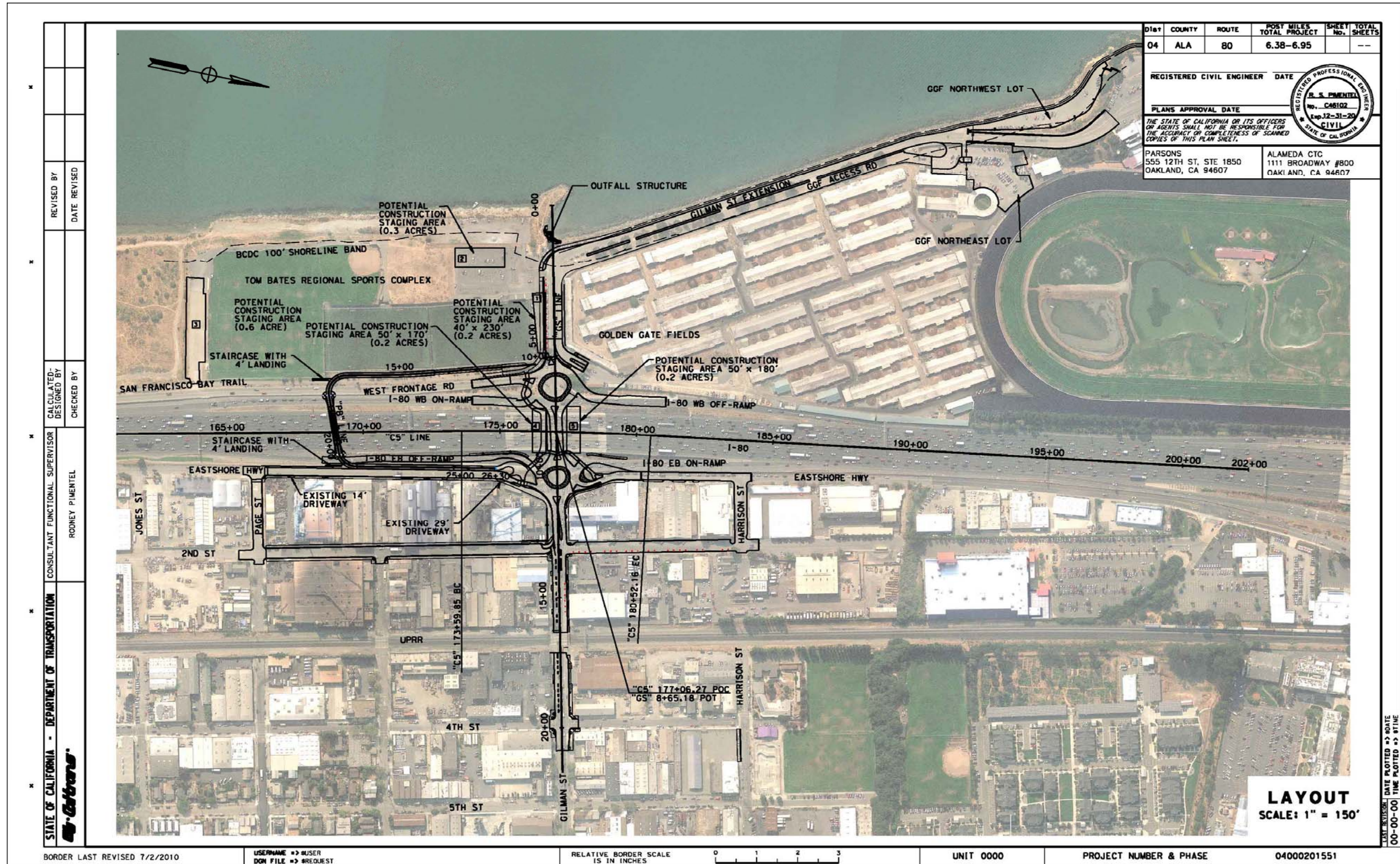
Figure 1-3: Build Alternative – Roundabout Alternative
